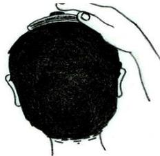
7. While holding steady in this position, gently press and release the set button located on top of the LaZee-Mouse. This is what sets the LaZee Mouse™ "home position". The home position is where the user returns to when no cursor movement is desired.
